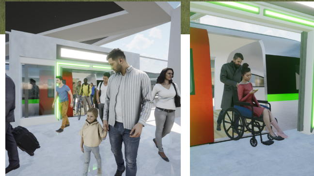
Level entry and exit.
